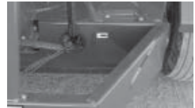
Transfer Auger Rear Bearings(2 remote zerks on rear of frame) Transmission Output Shaft Collar(1 remote zerk on rear of frame) Transmission Input Shaft Bearing(1 remote zerk on rear of frame)
